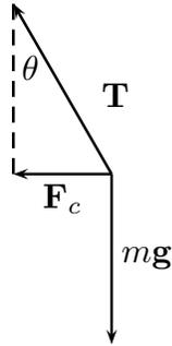
Since the mass is not accelerating up or down, the  $y$  component of the tension must be equal to the weight of the mass.
