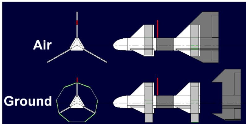
*Figure 7. Drop vehicle and ground rover.*
