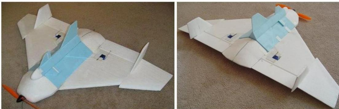
*Figure 2. Primary UAV and drop vehicle, 75 % subscale models.*
