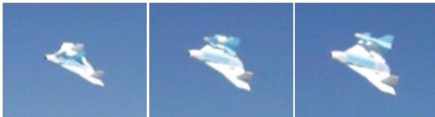
*Figure 9. Drop vehicle catching on vertical tail.*
