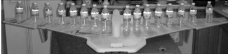
*Figure 6. Wing bending test*
